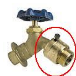
6.4 Item 1(Picture) recommend installation of vacuum breakers (anti-siphon device)
